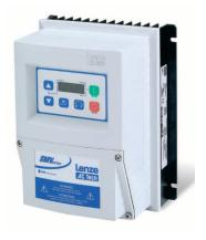
The new SMV range of IP65 inverter drives offer sophisticated auto-tuning, fast dynamic torque response with impressive low-speed operation all from a compact and simple to use package. Ingress protection to IP65 allows for use in outdoor applications and indoor environments where atmospheric moisture is present or low pressure water jets are used.
